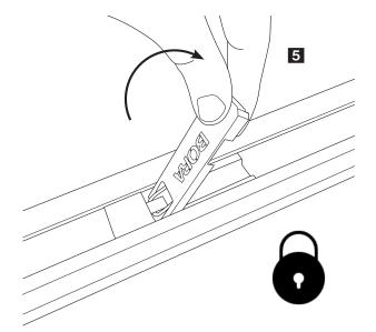
Clamp the Cutting Guide to the Material
