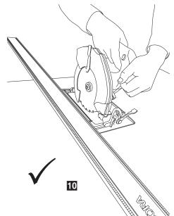
Recommended cut direction is from the sliding clamp toward the fixed clamping head.
