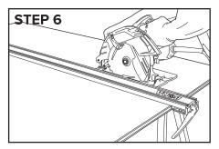
Check that the clamp is in the correct place and secure to do work. If adjustments need to be made repeat steps 3 to 5. Only cut when you are satisfied the clamp is in the correct position and you are ready to work.
