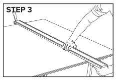
Move your guide to your work piece and pull the end clamp head so that it is 1" (25mm) wider than your material.
