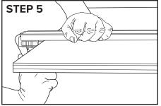
With both guide heads in place, push the clamp handle down. This will push the clamp head closest to you toward the head you placed in Step 4.
