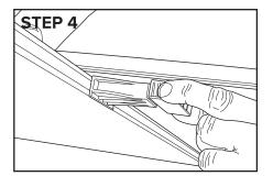
Now hold the clamp head between thumb and index finger as shown and push toward the material. Once this is in place you are ready to clamp.
