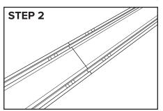
Connect the guide and the extension with the connectors supplied and tighten hardware.
