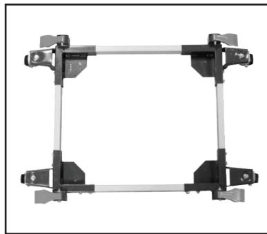
A short narrow base, such as found on a drill press or bandsaw may benefit from this arrangement. Due to swivel rotation, base may sit out of level. Rotate swivel wheel away from base to correct.
