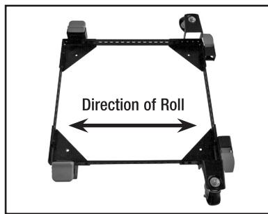
A short narrow base, such as found on a drill press or bandsaw may benefit from this arrangement. Due to swivel rotation, base may sit out of level. Rotate swivel wheel away from base to correct.
